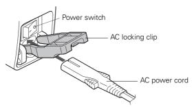
Plug the free end of the power cord into a power outlet.
